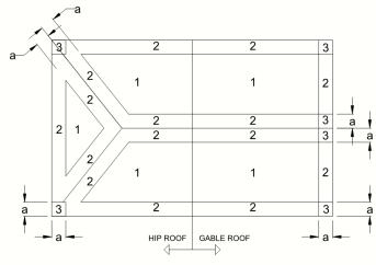
a: 10% OF LEAST HOIZONTAL DIMENSION OR 0.4h, WHICHEVER IS SMALLER, BUT NO LESS THAN EITHER 4% OF LEAST HORIZONTAL DIMENSION OR 3FT (0.9M).
